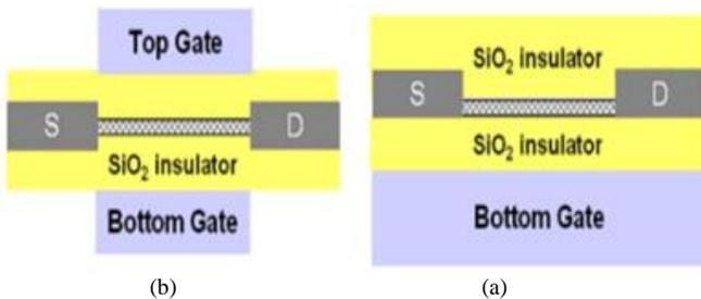
Fig 6: General schema a) graphene-based transistor with one gate b) graphene-based transistor with one gate [3].
