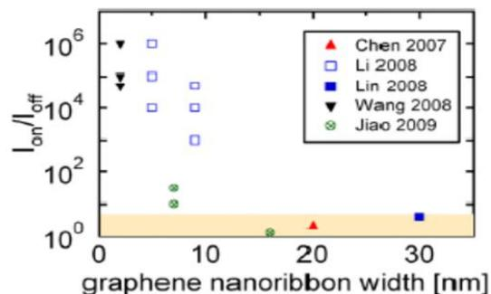
Fig 9:  $\frac{I_{on}}{I_{off}}$  ratios per bars width which are obtained experimentally [11].
