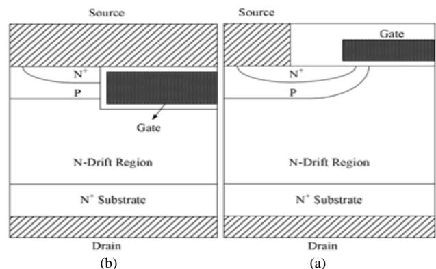
Fig 5: a) Vertical D-MOS transistor b) U-MOS transistor.
