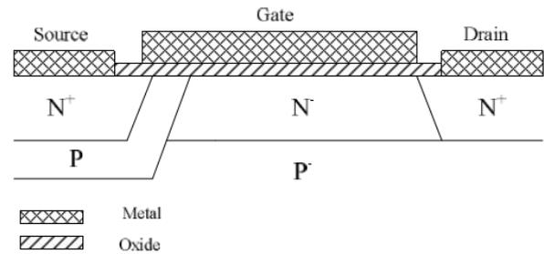
Fig 4: The structure of horizontal DMOS transistor.
