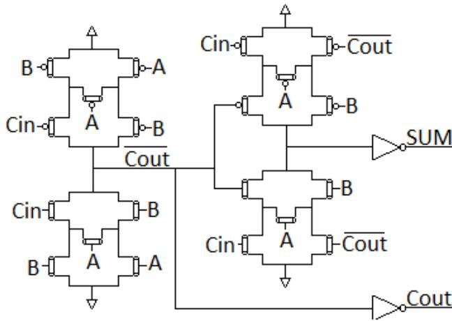
Fig 13: full adder circuit based on carbon nanotubes
