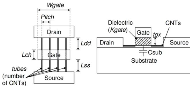
Fig 10: Side and top view of CNTFET transistor [5].
